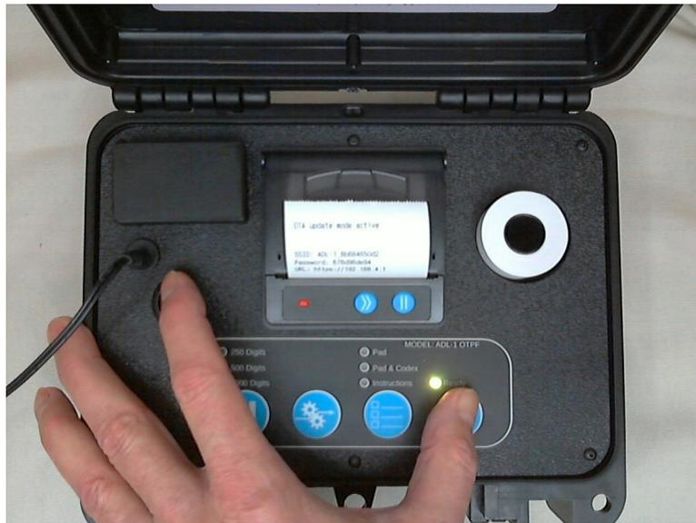
Tear off the printed WiFi connection information, leaving the printer powered on.
