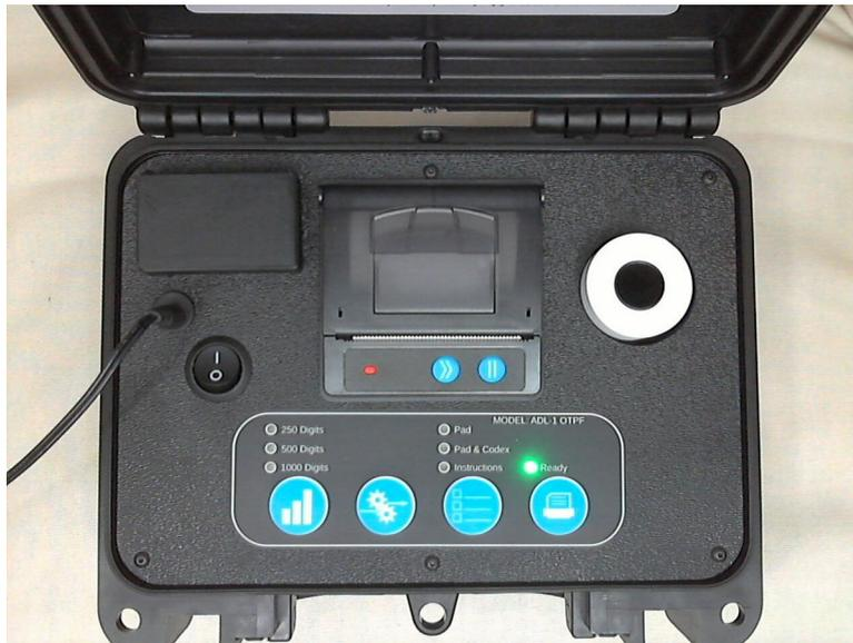
If your computer will not connect, try a different device. Power cycle the unit and repeat step 5, each time. There is only provision for 1 connection so it needs to be reset between attempts.
