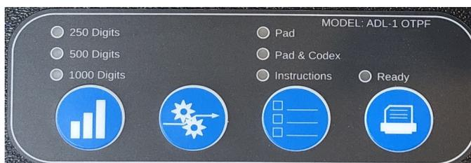
5. With the unit off, hold down the “Print” button and turn the unit on.
