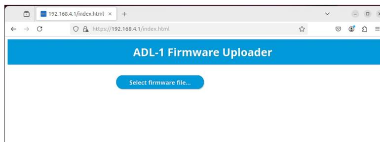
8. Press the “Select firmware file...” button and select the ‘A’ or ‘B’ firmware image as required. You will see this:
