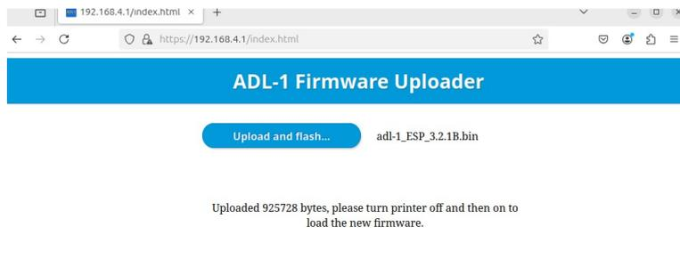
11. Turn off the printer, hold down the “Generate” button and turn the printer on. It will print the firmware version. Check it to make sure it matches what you just uploaded.
